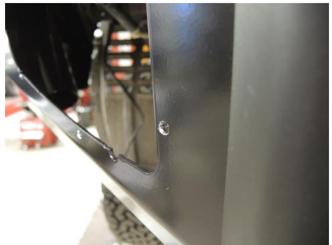
Paint holes to protect ( step 4 )
