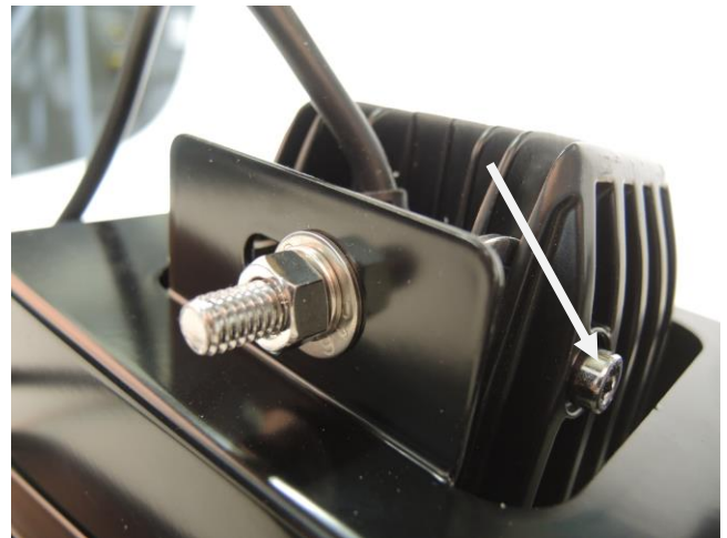
Note adjustment screw (Rigid LED) or see LED light manufactures instructions ( step 5B )
