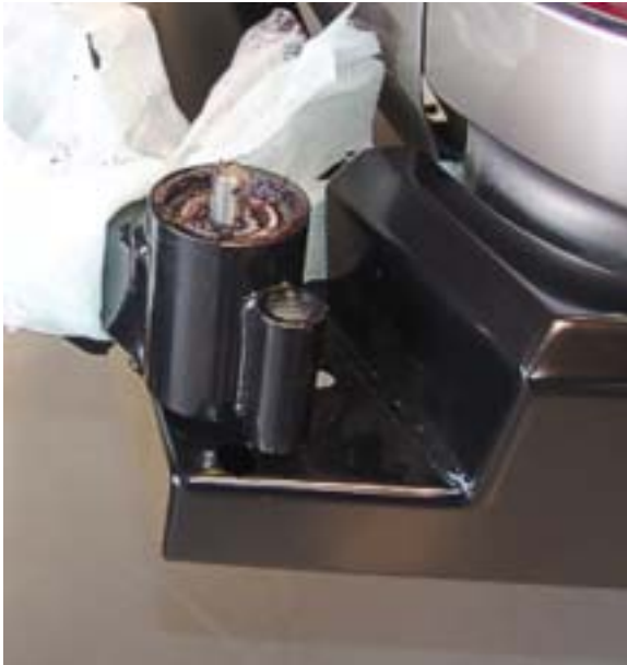
Tire Carrier installed on bumper.
