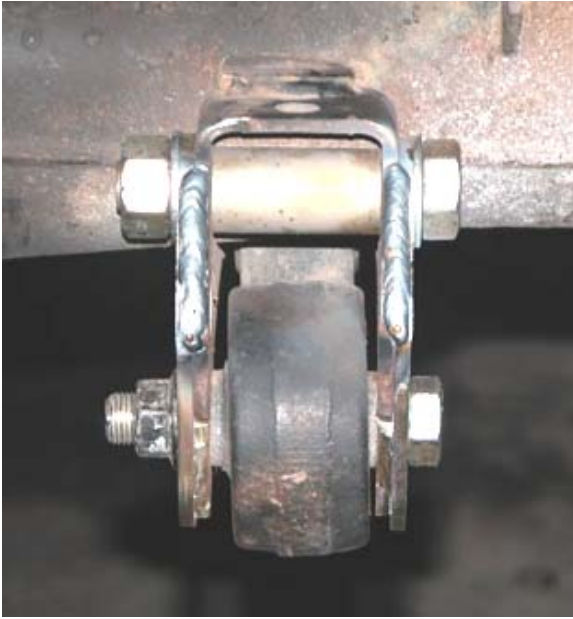
Driver Side Assembly showing sleeve in place and suggested welding.
