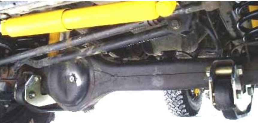
Reference picture of installed caster plates.
