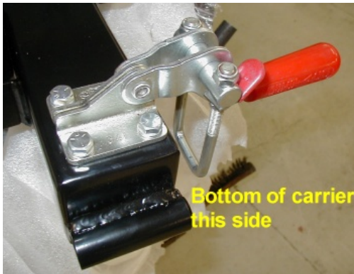
Tire carrier latch installed on tire carrier.
