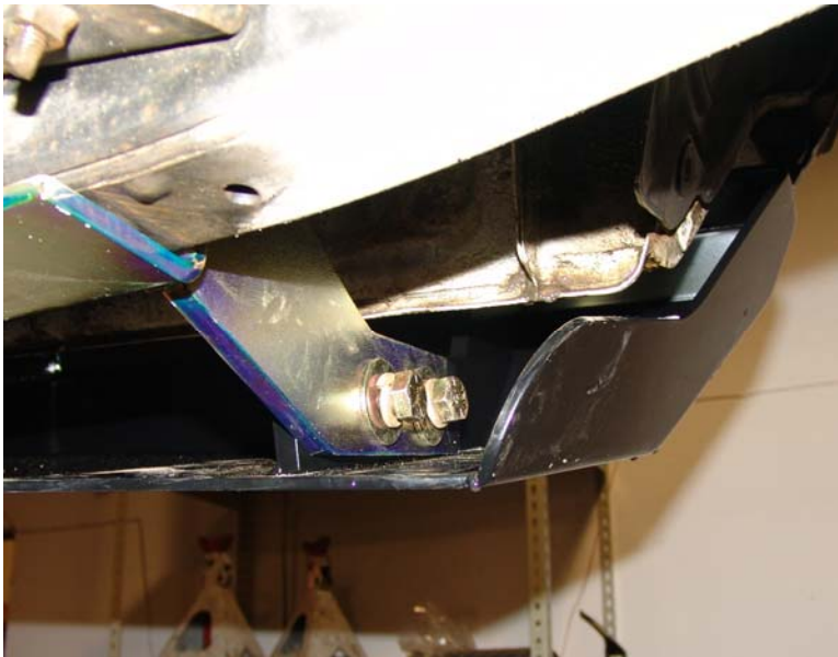
Driver side bracket bolts to bumper flange on the bumper.
