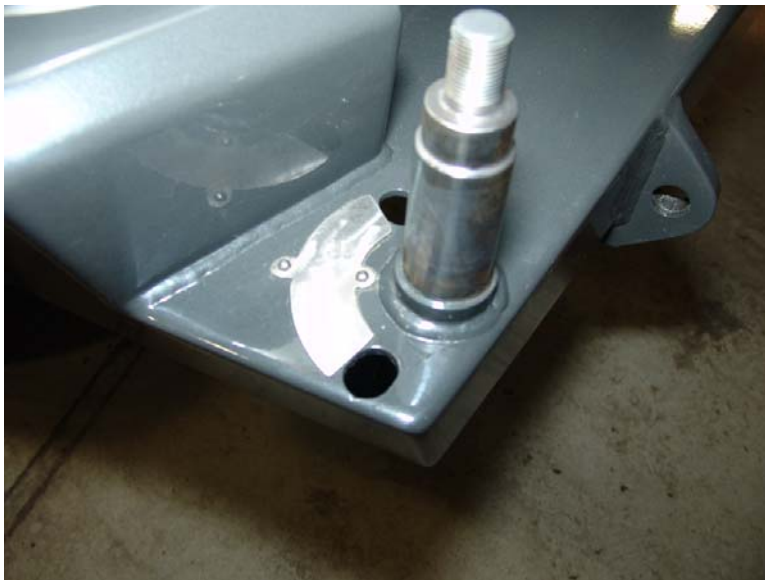
View of the slide strip installed. NOTE: This should be installed before the tire carrier is installed.
