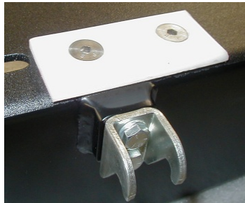
Nylon latch plate installed on top of bumper.
