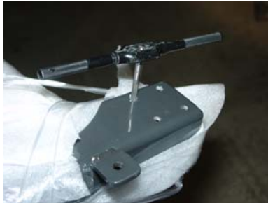
Tire carrier latch installed on tire carrier.
